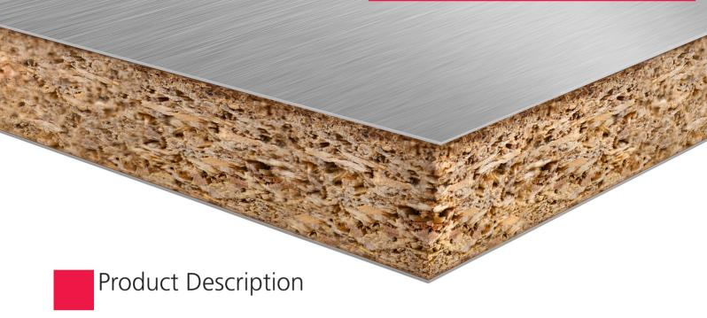
DekoSpan composite elements are high-quality panels with real metal surfaces (aluminum) that are applied to various substrates. The aluminum surface is permanently protected by a stove-enamel finish based on epoxy resin.
